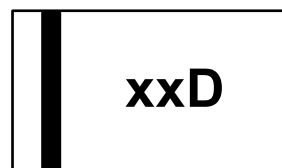
xxD: Device Marking Code Bar denotes Cathode
